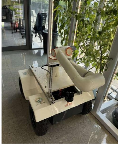
Figure 1 Fully assembled robotic harvesting platform
